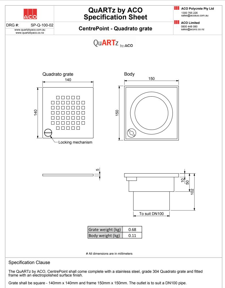
Grates shall be fastened with boltless mechanisms.
